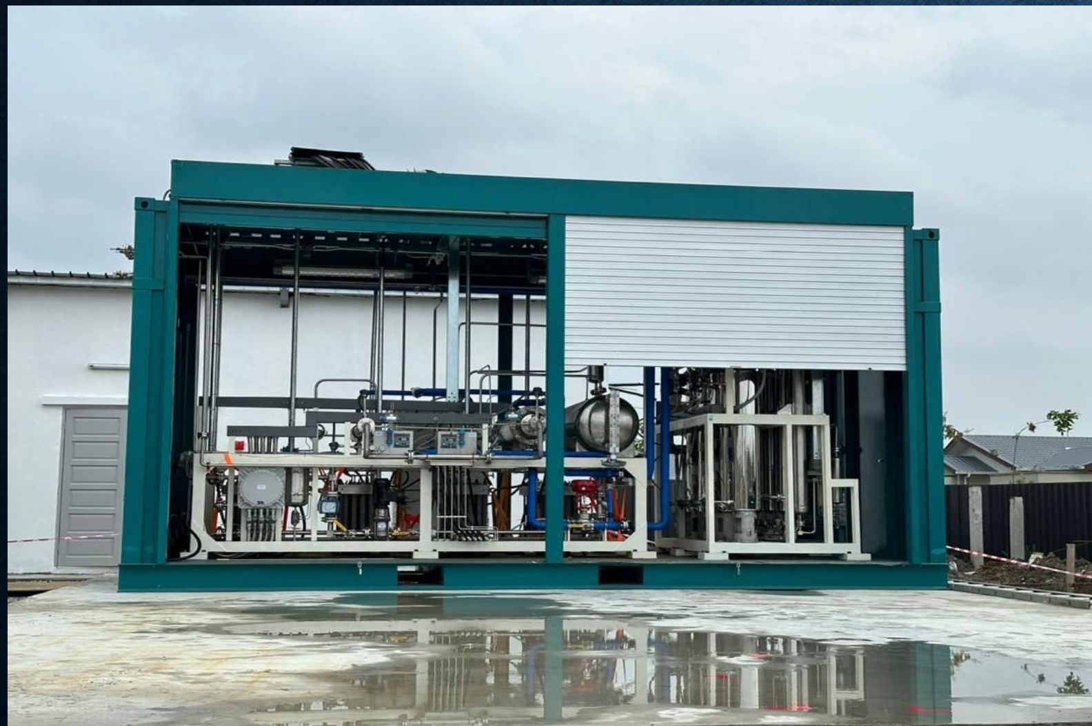
Electrolyser at Petros Multifuel Station Darul Hana
