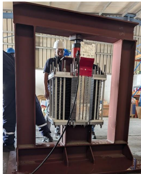
Compression of stack with hydraulic press
