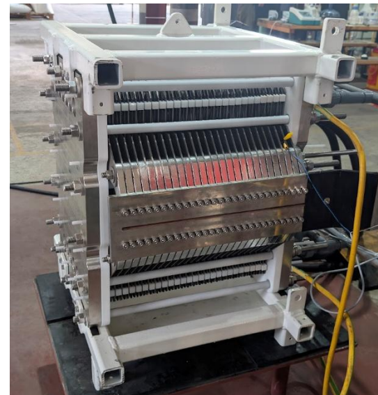
Fully assembled electrolyzer stack undergoing FAT
