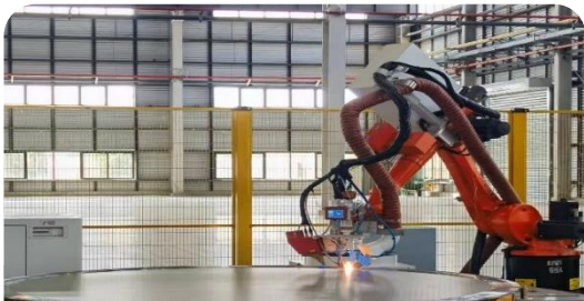
AI Vision V3.0 Weld Seam Tracking System, Real time Tracking Technology, Laser Weld Seam Adaptive Tracking and Focus Tracking Compensation
