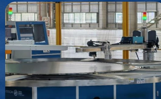
AI Visual Weld Quality Monitoring System Real time monitoring of electrode welding quality, abnormal alarm
