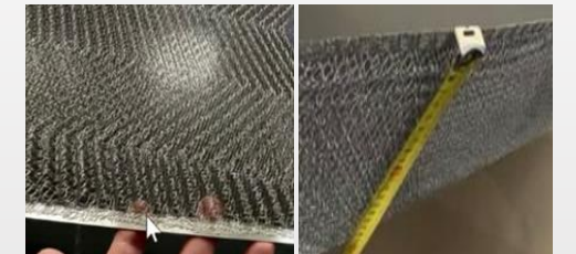
Plastic deformation or collapse
